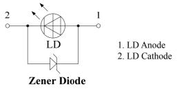
This model does not have a Photo Diode. This model has a Zener Diode built in as a protection circuit against static electricity.
