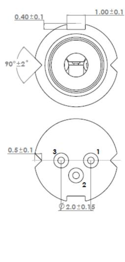
Note: Tolerance is  $\pm 0.05$ mm for items without tolerance marking
